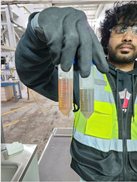
Photograph of Leachate Before (right) and After (left) Aclarity Process
